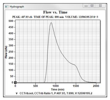
Figure 4 Solution hydrograph for HEC-1 Simulation
