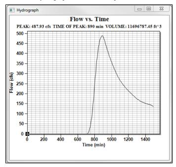
Figure 3 Hydrograph after first HEC-1 run
