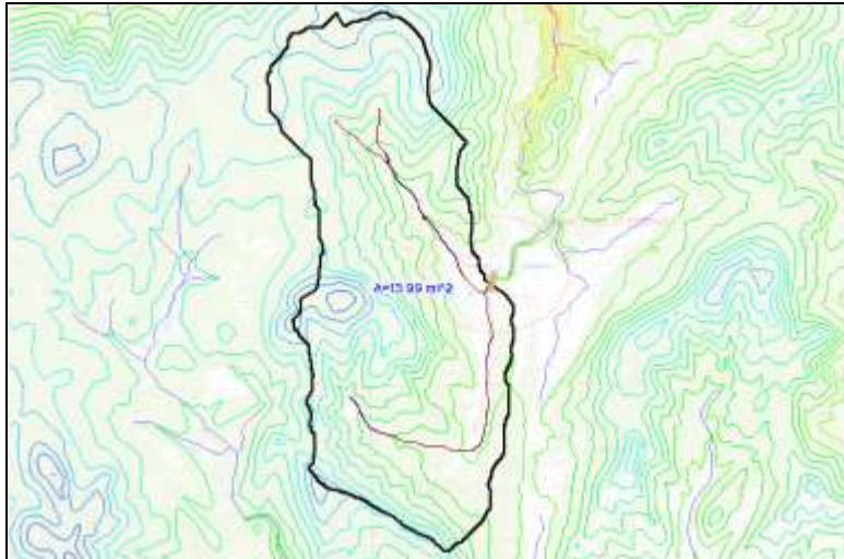
Figure 4 Delineated watershed with outlet at the culvert
